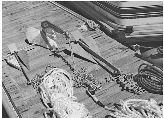
My anchor collection: a small Danforth with 12 feet of chain and 100 feet of nylon rode (left); a Delta plow with 15 feet of chain and 150 feet of nylon rode (center); another older, larger Danforth from a previous boat with about 15 feet of chain and 75 feet of rode (right).
