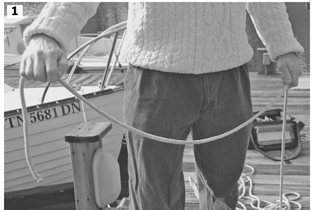
1 Coiling a line. Hold the line fixed in your right hand. Reach back a comfortable distance with your left hand—
