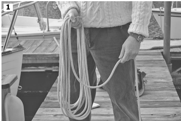
1 Securing a coil. Leave a few extra feet loose when coiling.
