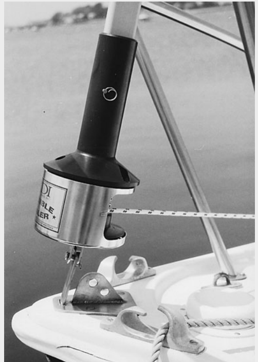
Typical roller-furling units small enough for use on a trailer sailer; left is a Schaefer unit; above is from CDI.
