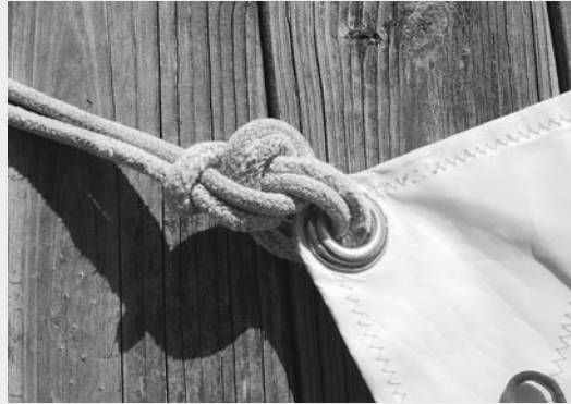
A bowline on a bight tied to a headsail.
