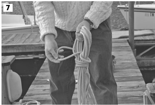
Securing a halyard on a cleat. Leave the coil open; don't take any turns around the entire bundle. Grab the middle of the loose end—
