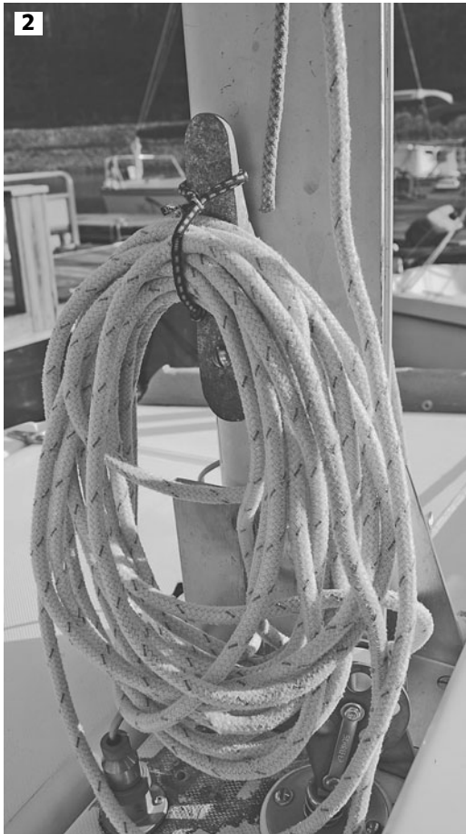
2 A halyard leash in use. The second loop fits over the upper horn of the cleat, and gravity does the rest.
