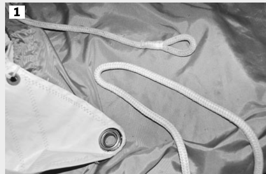
The Dutch shackle is really nothing more than a short length of line with an eye splice at one end. Here's how it's used to attach to headsail sheets.
