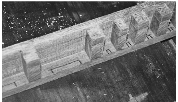
Step 4. Here the bottom rail is set in place; the small drain notches have been marked (left). All three pieces are shown (right).
