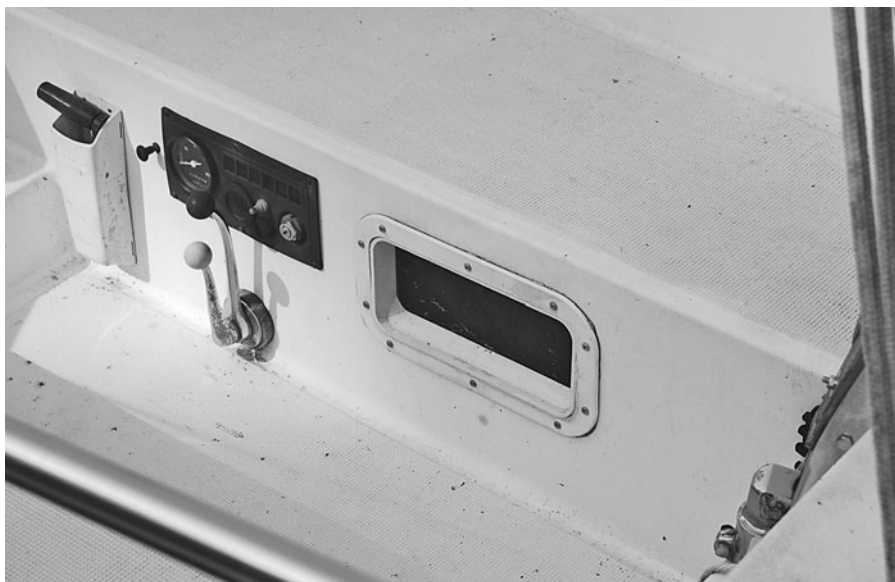
A plastic portlight used in the side of the footwell for ventilation and light. A clear inspection port works well, too.
