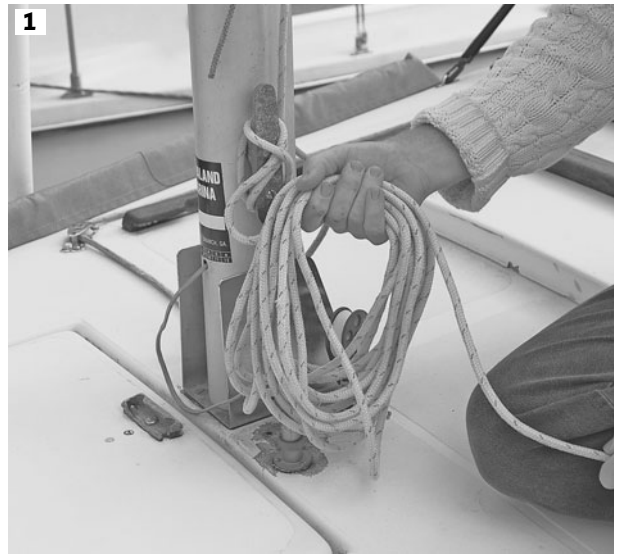
Securing a halyard on a cleat. Leave the coil open; don't take any turns around the entire bundle. Grab the middle of the loose end—
