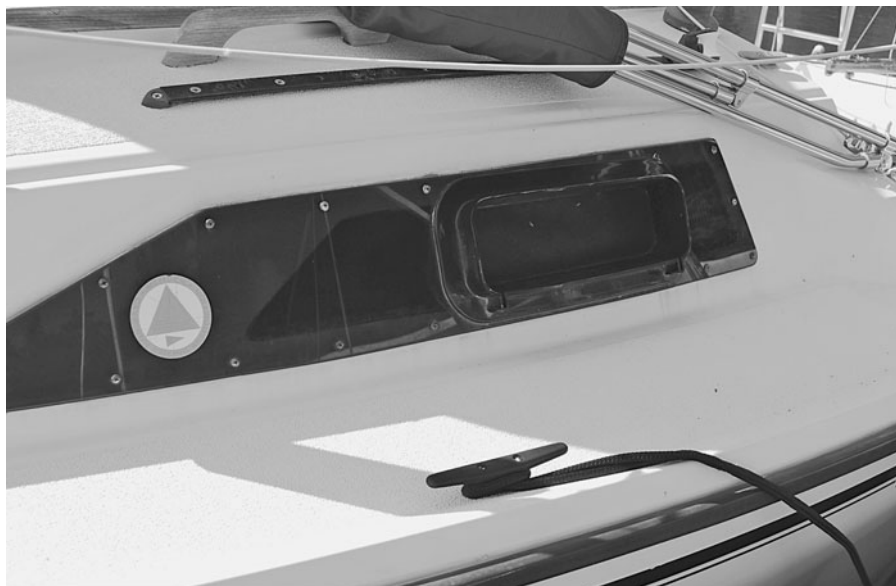
Opening plastic ports are factory installed in existing deadlights for improved ventilation. This black port in a smoked plexiglass deadlight is on a Precision 21.
