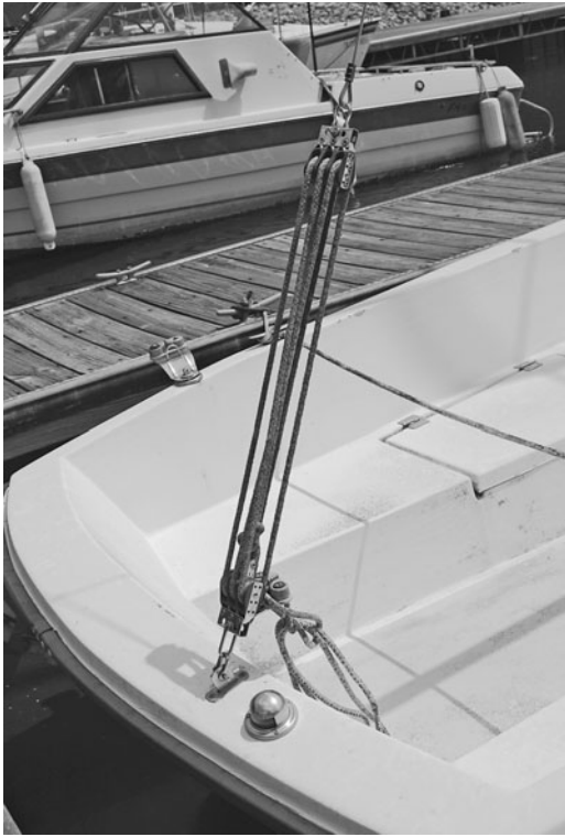
An adjustable backstay on an older boat. They are powerful blocks that can exert a lot of force on a rig. This particular one is a bad design—the only thing keeping the mast on the boat is that little cam cleat. If it were released accidentally on a run in a breeze, the entire rig could go overboard.
