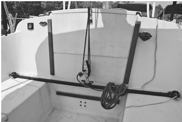
The traveler on my boat, while it is a handy and flexible sail adjustment, was expensive and is often tripped over when I'm going down below.
